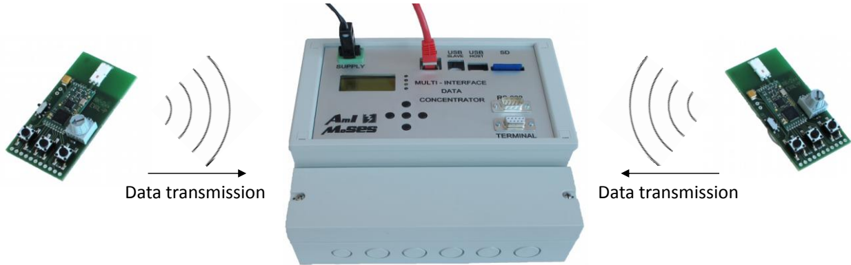
Figure 4: Prototype of Data Concentrator hardware unit and wireless AmI Data sources (temperature sensors)
