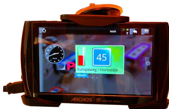
Figure 10 : The Android based EEIC on-board unit
