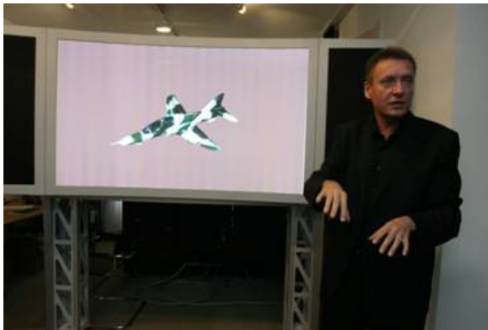
Figure 2. Large-scale HoloVizio light-field 3D display projecting 50Mpixels
