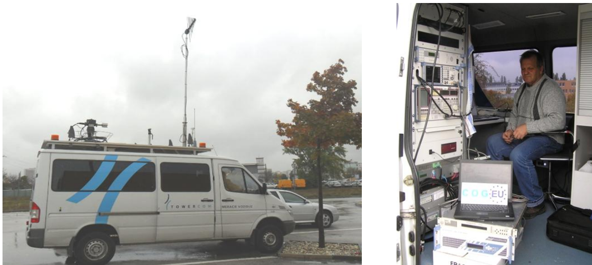
Figure 3 TOWERCOM's measurement van used in Bratislava city with a 5 m antenna height.
