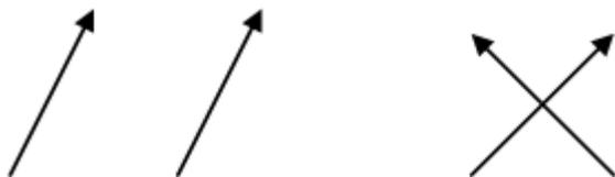
**Figure 2.4. Two antenna elements for conventional MIMO (left) and polarised MIMO (right).**
