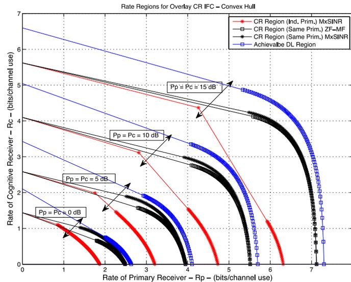
**Figure 2.2. Both CTx and CRx have 2 antennas each. For same primary message encoding strategy, rates have been plotted when CRx is ZF-MF and MxSINR. With independent encoding, ZF is not possible so MxSINR CRx is used.**
