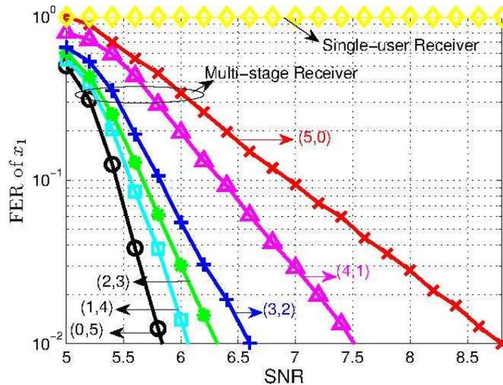
**Figure 3.3. Multi-stage receiver at CCS to detect  $x_1$ . (a, b) indicates splitting of interferences into groups where a indicates the number of interferences in the first group (linear receiver) while b indicates the number of interferences in the second group (non-linear ML receiver). Alphabets belong to QPSK and SNR is the received SNR at CRx1.**
