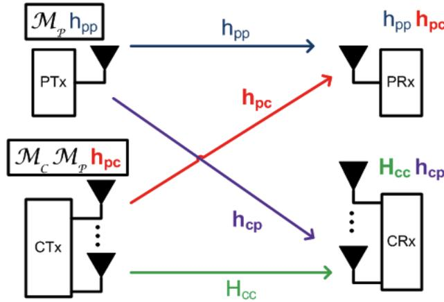
Figure 2.1. System model for 2-user cognitive radio interference channel.
