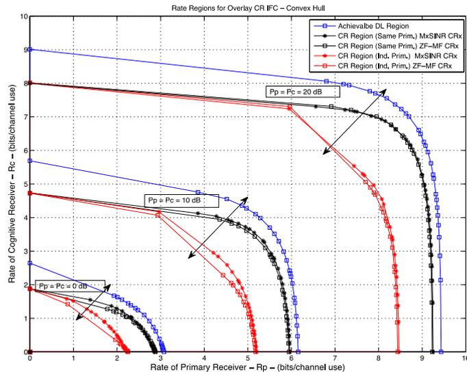
**Figure 2.3. Both CTx and CRx have 3 antennas each. The rate regions have been plotted for both schemes when CRx employs Mx-SINR and ZF-MF receiver. MxSINR receivers bring some gains over ZF-MF for lower power constraints.**
