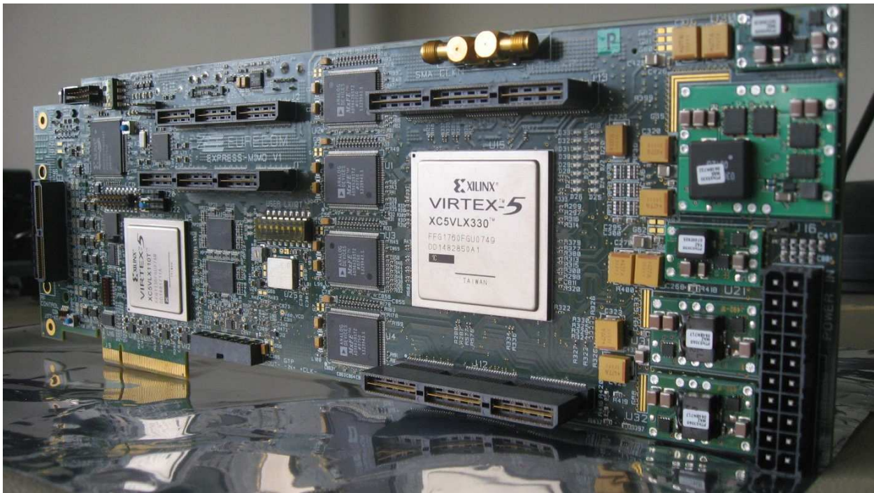
Figure 3-11: The ExpressMIMO board
