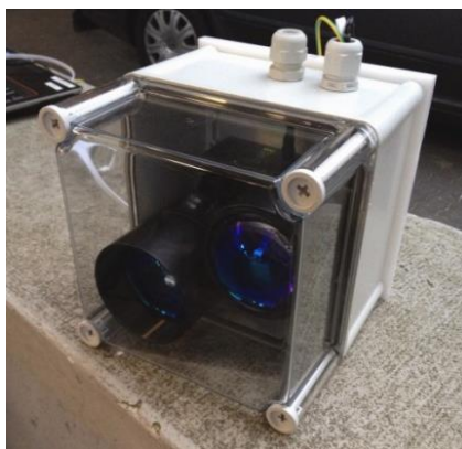
Figure 7: Left: Optical wireless transceiver prepared for outdoor trials. Right: Campus map of TUB where the link is installed (source Google Earth/Berlin 3D).
