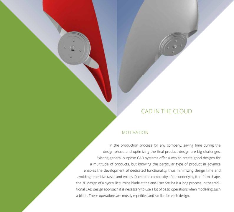
The goal of this case study is to reduce the amount of time needed to design a popular blade type called Kaplan blade. In Stellba's case, such a design process happens typically bi-weekly. An additional goal is to save, manage and share data by using the Cloud and a Cloud-based PLM system.
