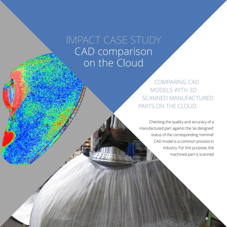
with a 3D acquisition device, e.g. a laser scanner, which results in several point clouds typically consisting of millions of measured, discrete 3D points. To determine where deviations between the CAD model and the point cloud exist, the two data sets need to be aligned and matched in a process called registration and distances between the closest points of both models need to be calculated.
