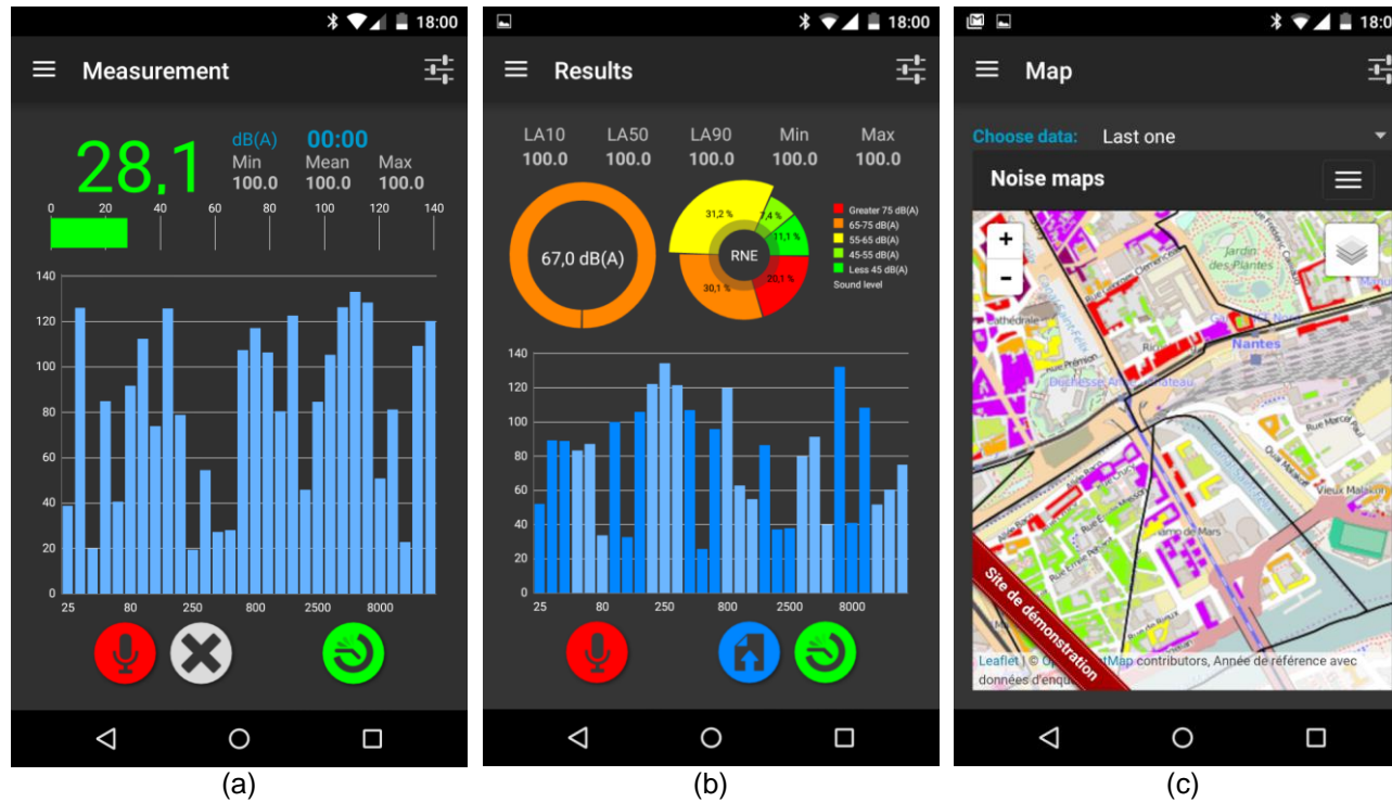
Figure 5: Screenshots of the NoiseCapture application: (a) measurement screen, (b) results screen and (c) noise map visualization.
