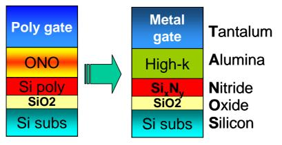
The most promising option to overcome these scaling limitations, while retaining the very high integration density of NAND Flash architecture seems to be the replacement of the conventional floating gate with a charge trapping layer. Even if apparently a direct evolution of conventional approach, the TANOS architecture implies introduction of new the
