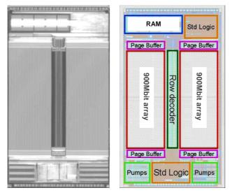
A 1 Gbit NAND memory device was modified by Numonyx to become compatible with the new cell architecture and fully functional samples have been obtained.
