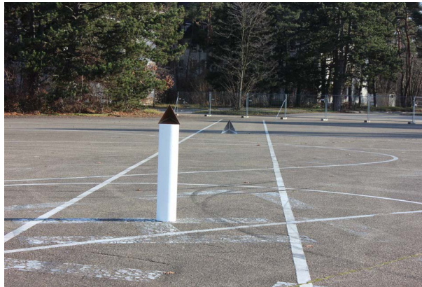
Fig. 3-1: Two corner reflectors in a distance of 30 and 60m from the radar
