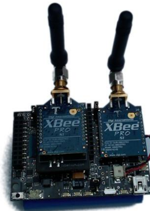
Figure 35: Waspnote node with 2 transceivers
