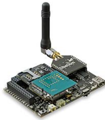
Figure 32: Wasmote communication module
