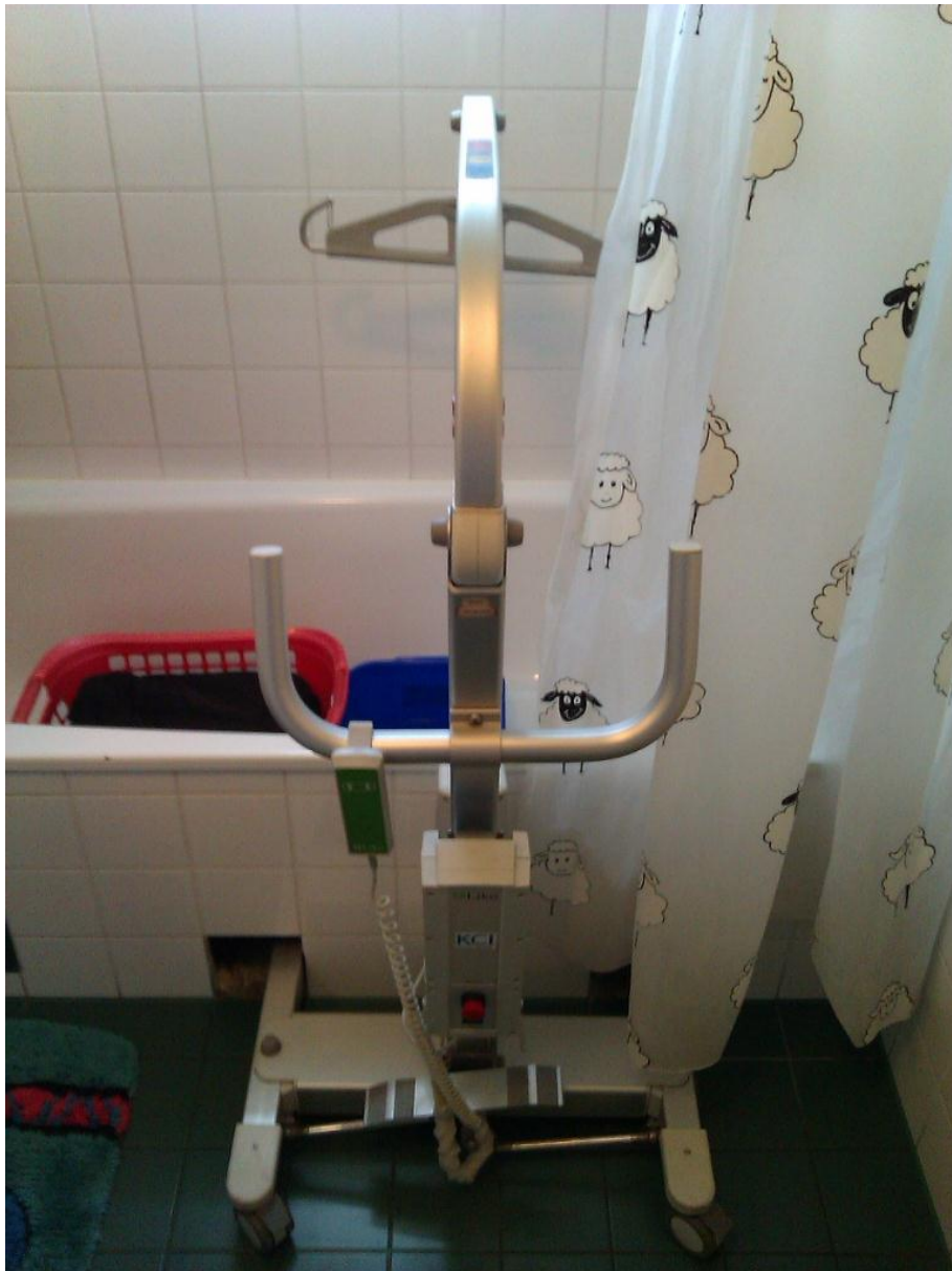
Figure 5: Bathroom of the end-user. This picture shows the lifting aid operated by the attendant by using the green remote control. The patient is moved on a swing made out of robust bandages fixed on the front of the lifter.
