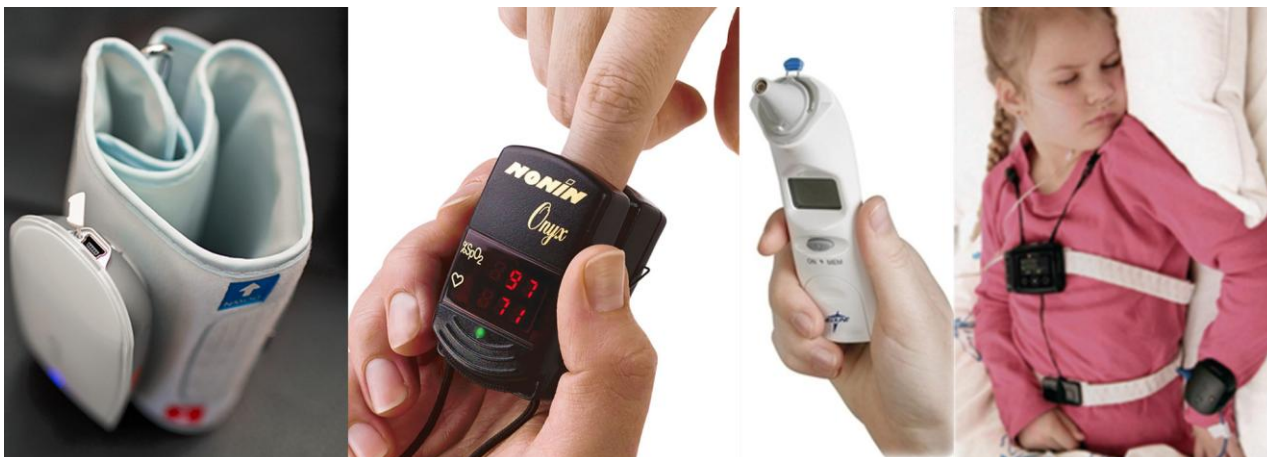
Figure 23: Possible sensors. Left: Wrist blood pressure (BP) monitor. Middle-left: Pulse Oximeter measuring pulse rate (PR) and arterial oxyhemoglobin saturation (SpO2). Middle-Right: Thermometer (BT sensor) Right: RIP belt - Respiratory Inductance Plethysmography belt – for measuring breathing patterns. The presented devices are examples only. The planned tender will determine the exact products to be used. More information: see annex.
