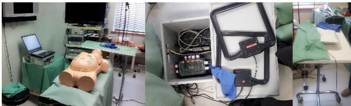
Figure 85: Left: OperationRoomManager laboratory with reporting station to the left, patient bed in the front, and Mayo stand to the back. Middle: data acquisition system to the left with 2 RFID antennas and one towel to the right. Right: RFID antenna on Mayo stand with towel and with towel package.
