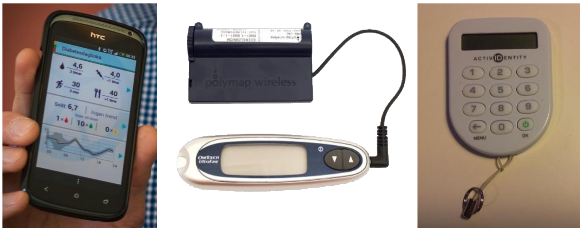
Figure 9: Smartphone with Diabetes Diary application (left) Lifescan UltraEasy glucose meter with a Polytel Glucose Meter Accessory (GMA) (middle), an Activ ID Entity authenticator device for generation of one time passwords (right).
