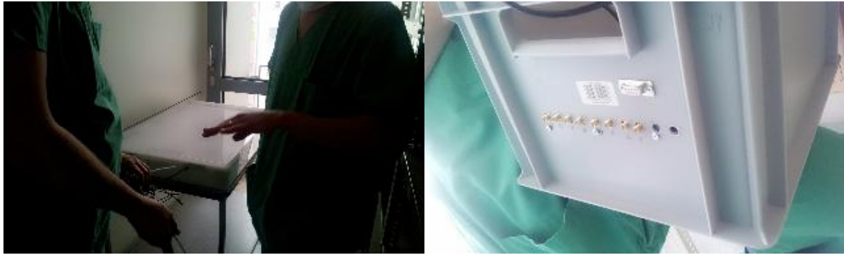
Figure 86: Left: Mayo stand fixture with integrated RFID antenna. Right: physical interface of RFID acquisition box for connecting antennas and the OTM PC.
