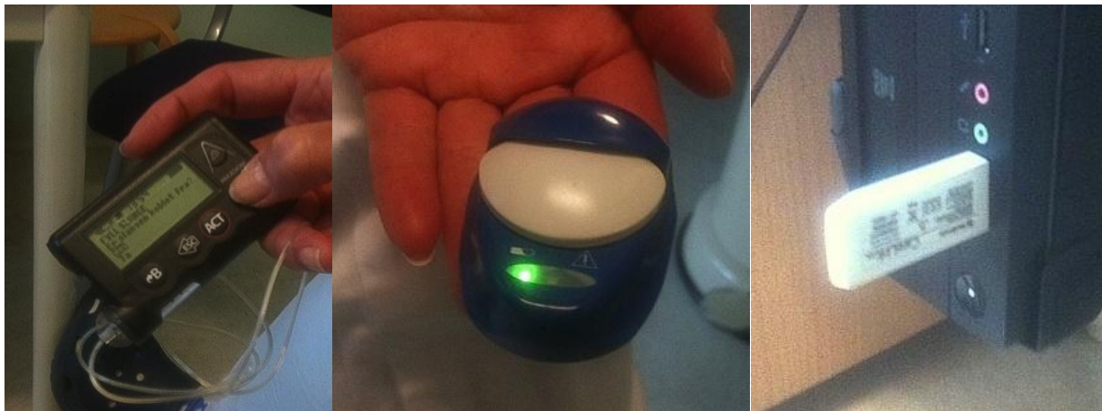
Figure 11: Medtronic Continuous Glucose Meter (left), a Medtronic wearable sensor (white) with charger (blue) (middle), a Medtronic USB communication-dongle (right).
