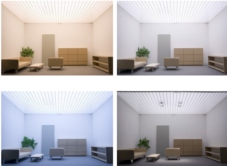
Fig. 5.1: Series F (residential) comparison; 3000 K (top left), 4000 K (top right), 6500 K (bottom left), 4000 K with TLM (bottom right)
