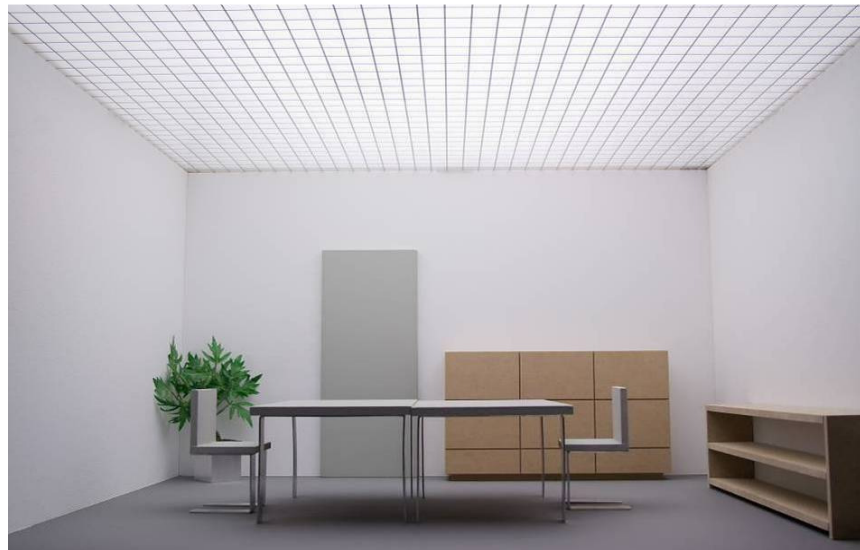
Fig. 3.23: Office room model with an OLED ceiling luminance of 300 cd/m 2 , OLED tile size is 15 x 15 cm 2
