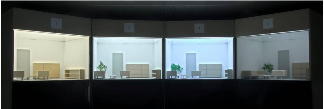
Fig. 3.28: Four room models with different scenarios for comparative evaluation placed next to each other. In this case the colour temperature of light was altered which was subject of evaluation in another study. Details of this study are described in chapter 5.
