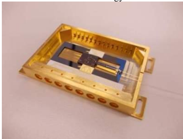
Figure 23: Assembly of the Rx model in the metal housing and connections to the primary RF ceramic PCB.
