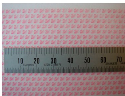
Fig. 10: Over-printing, wet-in-wet, large (about 2 x 3 mm) flexo patterns. Left, first printing pass. Right, 20 th printing pass.
