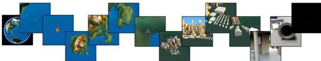
Figure 1. Navigation between scales in 3D scenes. Here, the user navigates from thousands of kilometres above the Earth’s surface to come to rest inside a jug on a table only centimetres in diameter. Note the smooth change in the vertical direction as the view approaches ground level. (McCrae et al., 2009)
