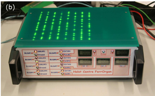
Figure 17: (a) Bench set-up for memory matrix array testing and characterization, (b) picture of "FerrOrgan" and (c) screenshot of (part) of the Labview software.
