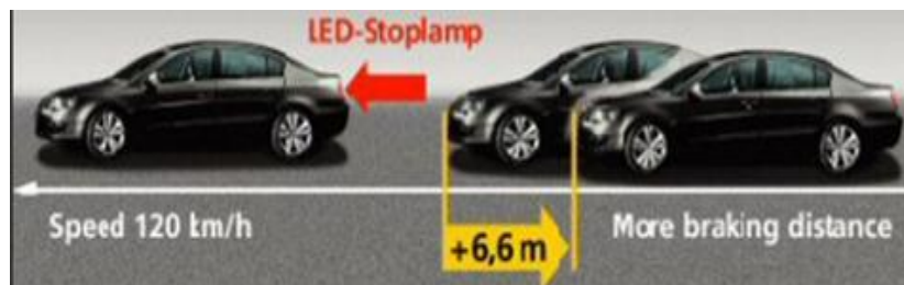
Figure 9 - Increased safety when braking (AL courtesy)
