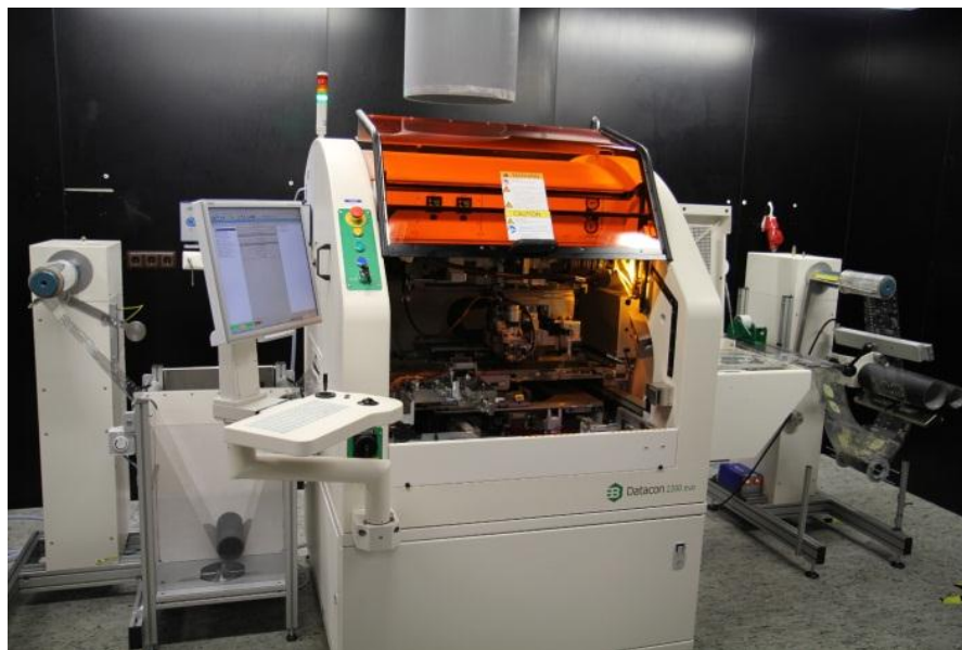
Figure 27 - Datacon EVO 2200 R2R bonding machine
