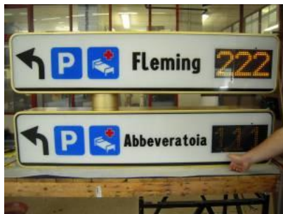
Figure 6 - Parking indicators printed and LEDs
