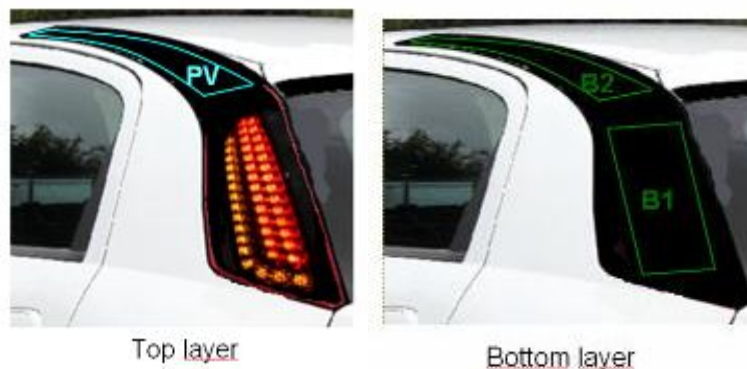
Figure 19 - architecture of the rear combination lamp
