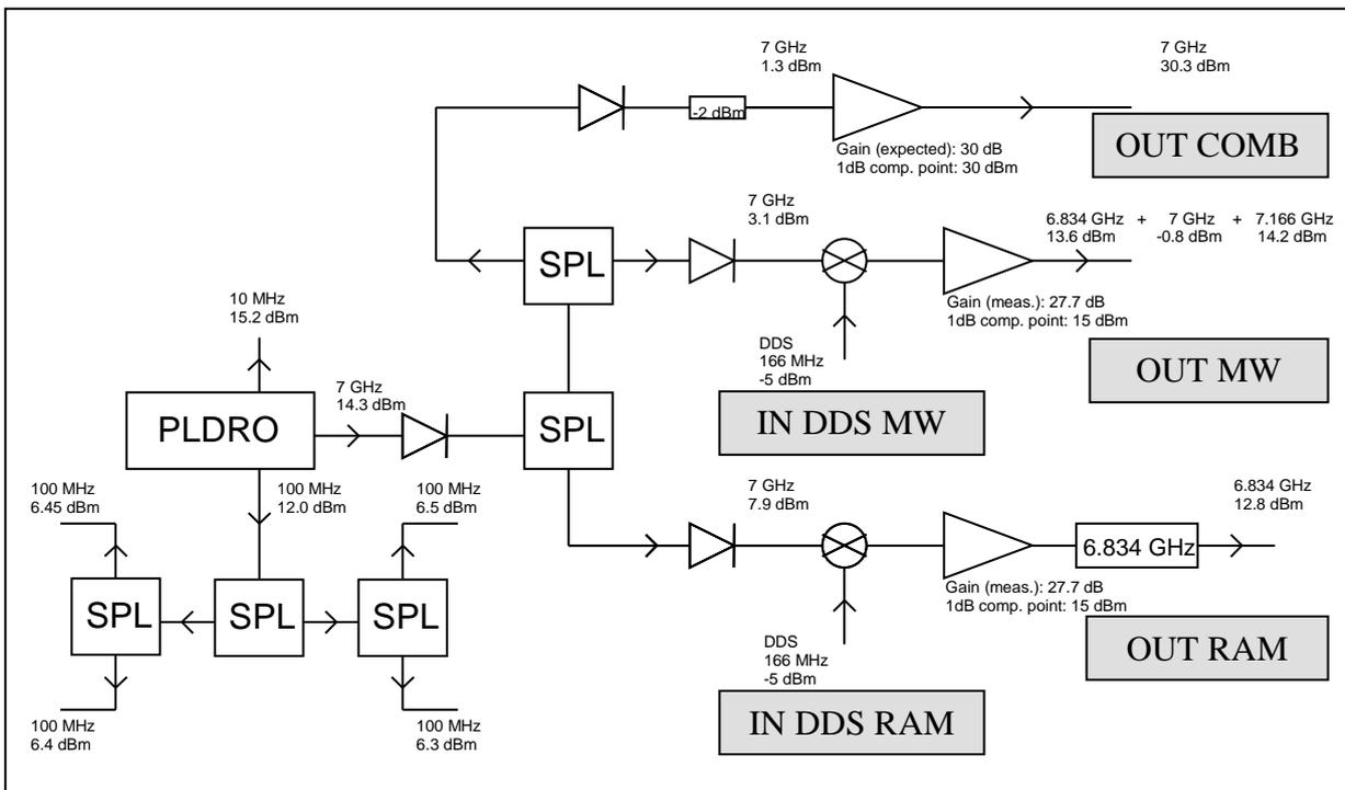
Fig.1 - Schematics of the PLDRO microwave chain
