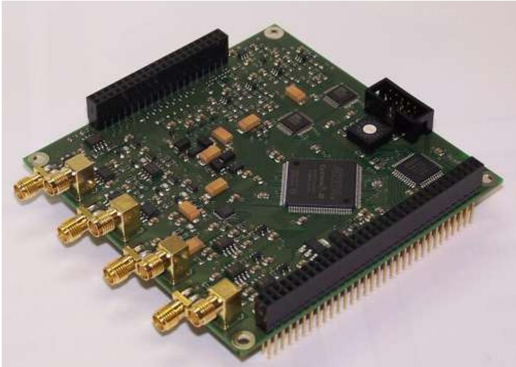
Figure 30: FPGA based frequency controller
