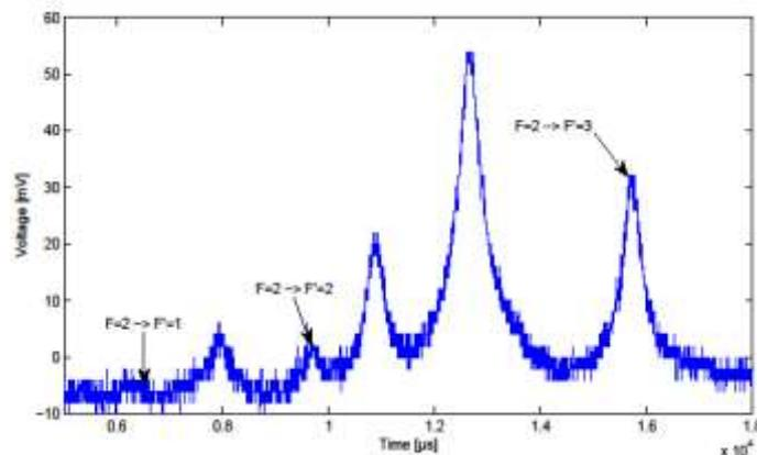
Figure 32:  $^{87}\text{Rb}$  D2 line spectrum obtained using the LUH electronics delivered to Bham. The transitions  $F=2 - F'=1$ ,  $F=2 - F'=2$  and  $F=2 - F'=3$  are labelled.
