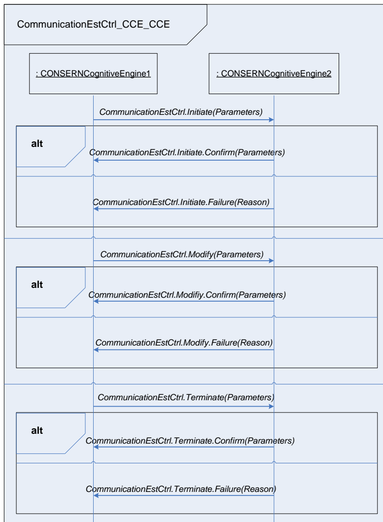
Figure 8-6: Service for Establishment and Control of a data link between two CONSERN Cognitive Engines.
