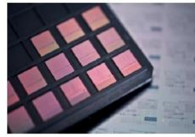
Left to right, diced Si photonic-IC wafer, chips ready to be shipped, Si photonic chip being packaged with fibre optic access ports.
