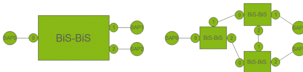
Figure 71: Illustration of the resource abstraction model BiS-BiS from the UNIFY project [30] and two levels of abstraction.
