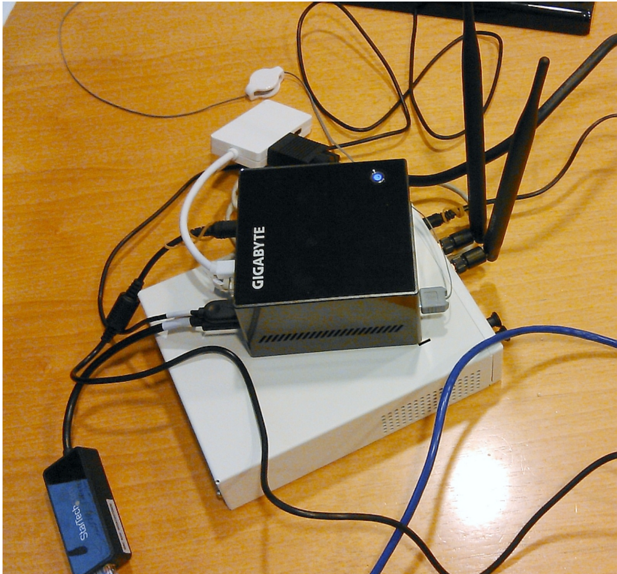
Figure 28: Mini PC running the LTE EPC + ENB software (on top) and an USRP N210 radio head (at the bottom)
