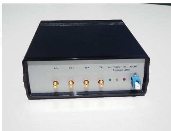
Figure 21: Photo of the 10 Gb/s ONU, which terminates the WDM-PON system and allows connection to various test equipment by SMA connectors.
