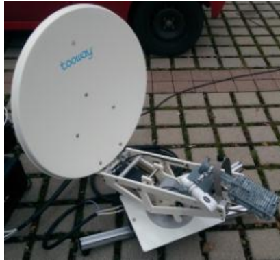
Figure 3: Deployable Ka-band satellite terminal
