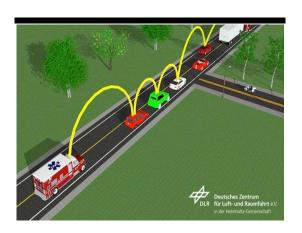
This in-car module allows wireless communication from vehicle to vehicle. Traffic management centres may receive event data or send traffic quidance information to the vehicle displays. This offers a scalable and independent transmissible solution by using a combination of proven in-car technologies,
