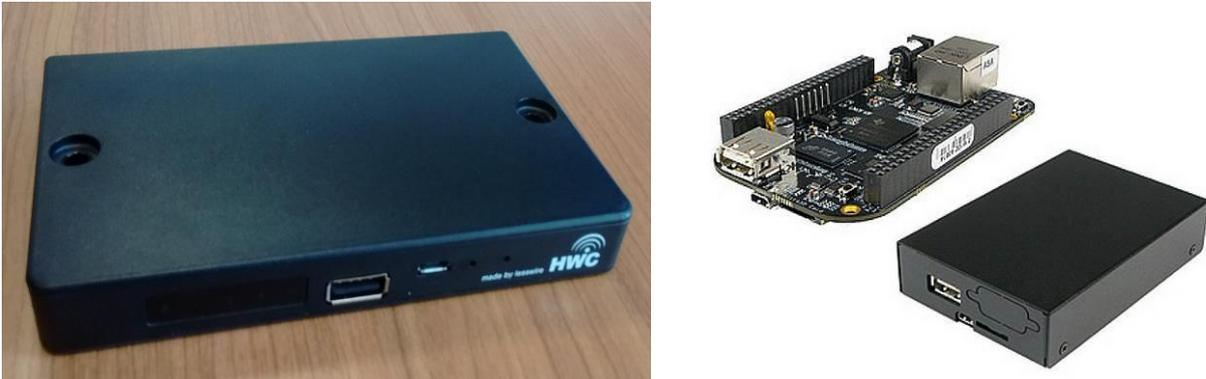
**Figure 12: Devices running the energy management algorithms and hosting the GUI web app. Left: HomeWaveControl. Right: Beaglebone black**
