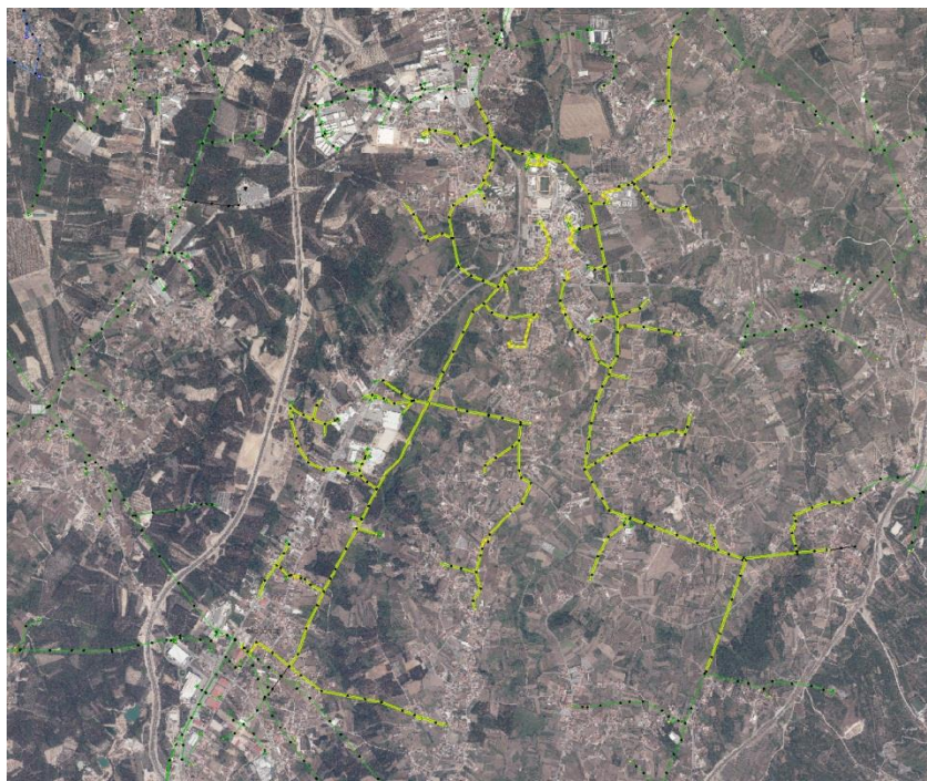
Figure 2: MV feeder (yellow)
