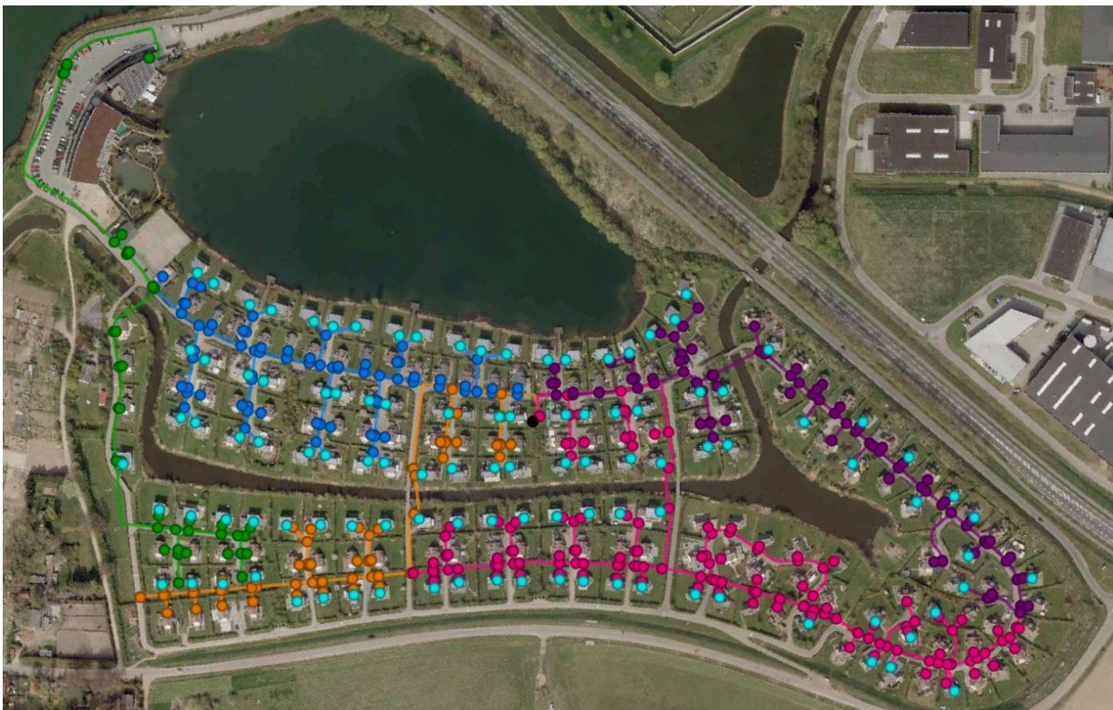
Figure 5: Aerial photo of the Bronsbergen demonstrator, with a LV-grid overlay. Locations of PV panels indicated by cyan coloured circles
