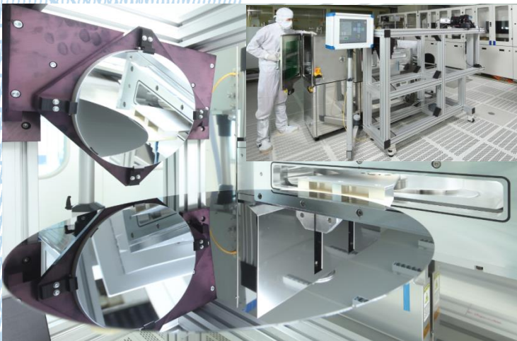
Figure 1: High-speed optical mapping and monitoring tool for 450 mm wafer diameter
