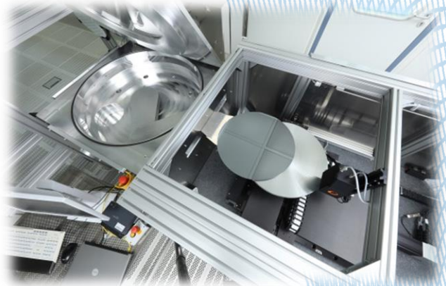
Figure: Open platform for metrology component evaluation that comprises a 300/450 mm transport tool and a versatile metrology module
