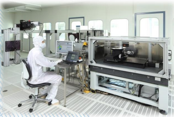
Figure: Open platform for metrology component evaluation that comprises a 300/450 mm transport tool and a versatile metrology module
