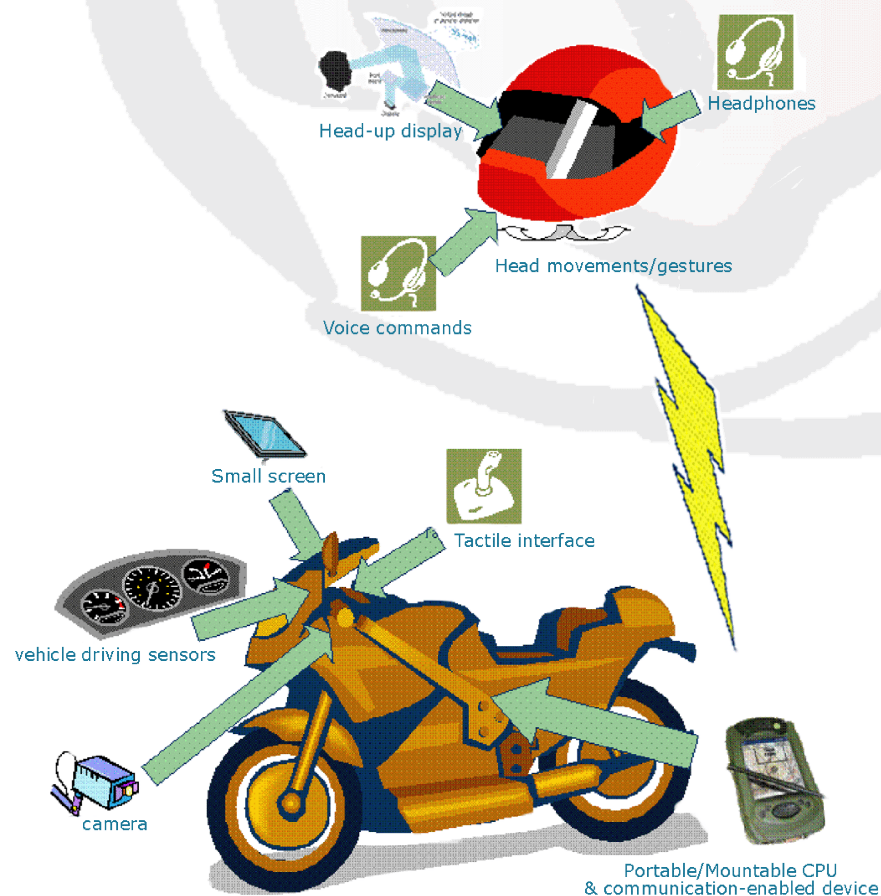
MoveOn environment: Multi-modal/multi-sensor helmet, robust speech-processing system, Police application
