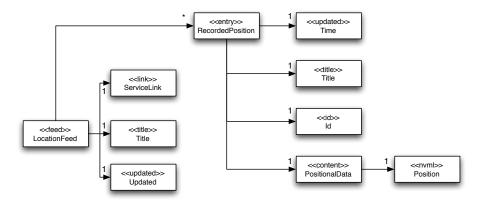
Figure 4.2: Positional Service Metadata in ATOM
