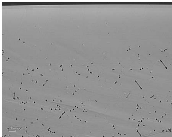
Fig 1: Defect etched bulk wafer illustrating oxygen precipitate induced stacking faults in wafer bulk.
