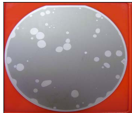
Fig.1: Germanium to sapphire room temperature bond interface.
