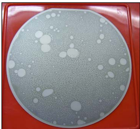
Fig. 2: Germanium/sapphire bond interface after anneal at 500°C.
