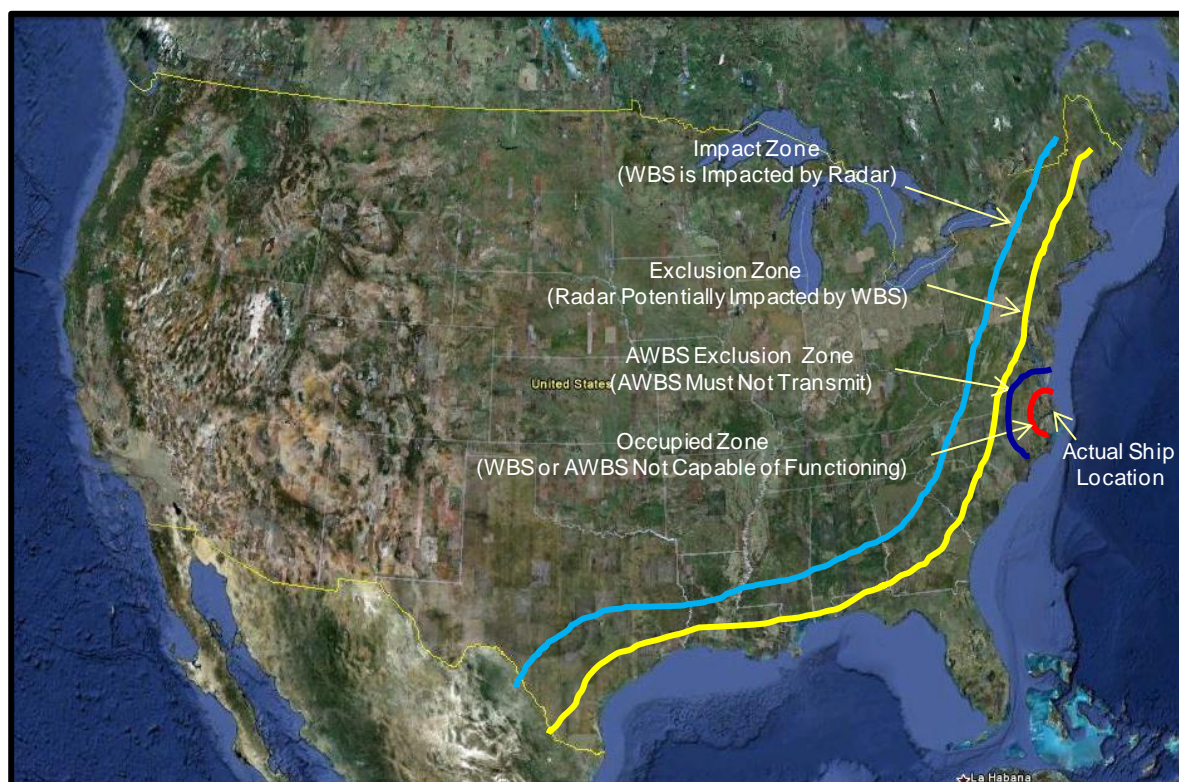
Figure 15: An example of secondary use of spectrum used by ship-borne radars, as being discussed in the United States [44].
