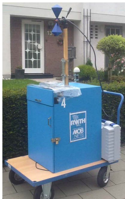
Figure 4-2 Measurement setup with mechanical tilting mechanism, mounted on wooden mast.
