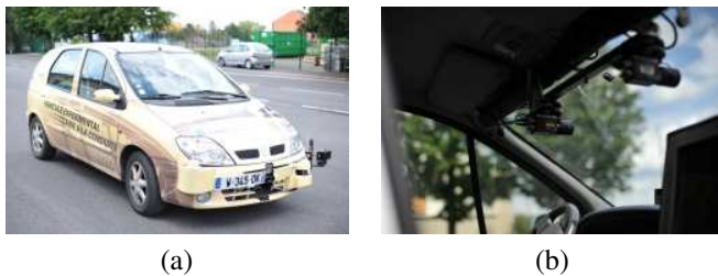
Fig. 13. Overview of the proposed system (a) instrumented vehicle (b) stereovision configuration.
