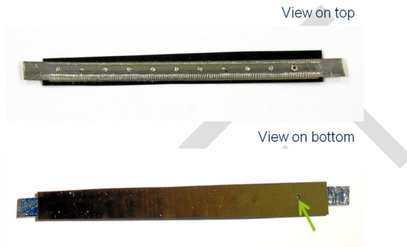
Fig. 3: Sample with established spot joints in the qualities: 2. Joint and 3. Hole (right, arrow)
