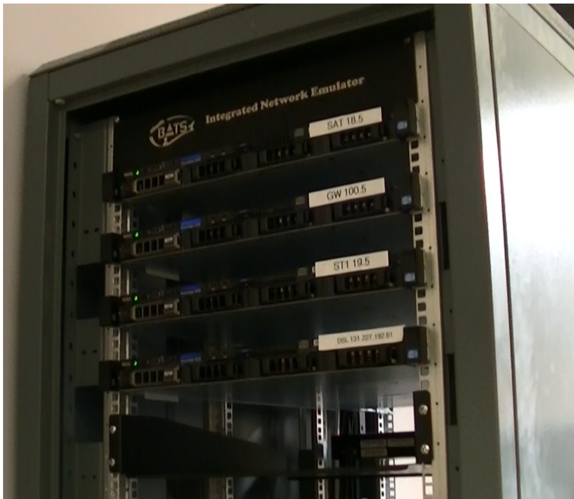
Figure 2-5 The OpenSAND and DSL transmission path emulators
