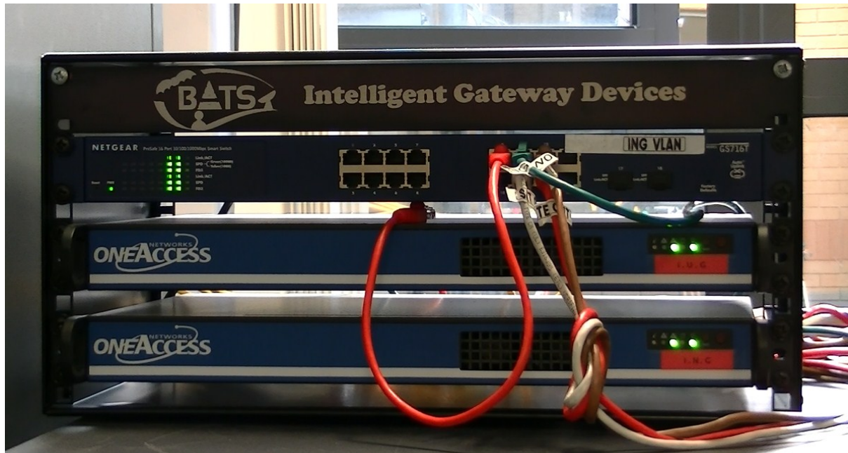
Figure 2-6 The IUG, ING and associated VLAN switch
