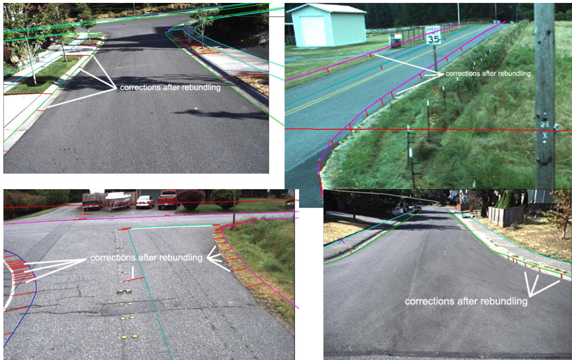
Figure 2: A selection of different crossings from a GeoAutomation dataset (Snohomish), the drift of the original measurements is clearly visible. The red correction lines indicate how these measurements will be repositioned after re-bundling.
