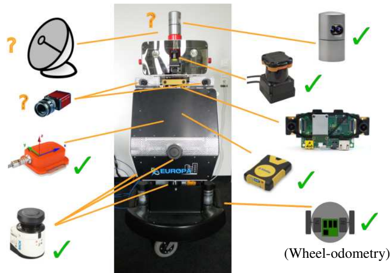
Figure 1: EUROPA2 sensor setup. The green checks indicate which sensor is already running in the EUROPA2 configuration on the ETHZ platform. The question marks indicate sensors or sensor placement, which have not been specified yet.
