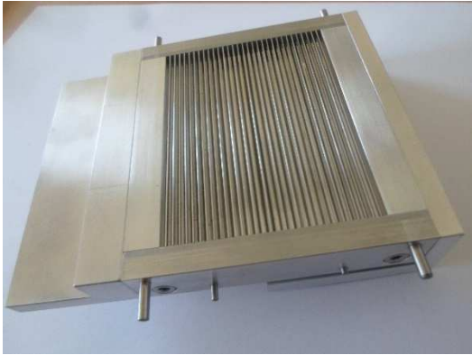
Figure 16 CTS antenna for backhaul link in E-band (left) and zoom on the switch component (right).
