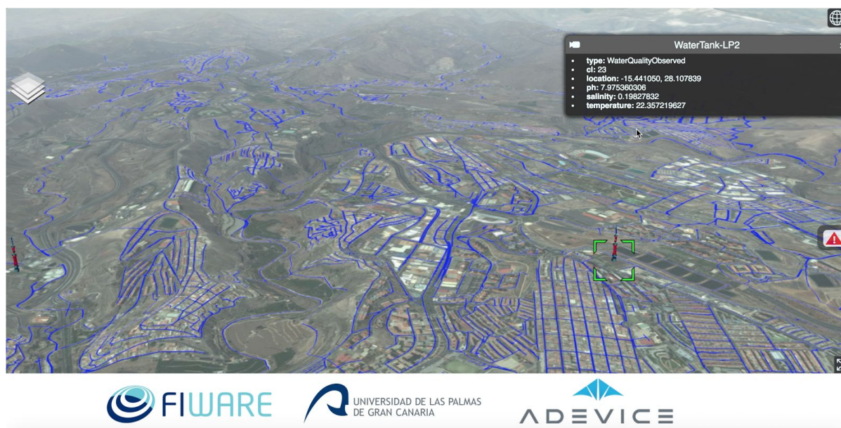
Figure 7.- View of the web application with the wastewater network loaded displaying sensor data.
