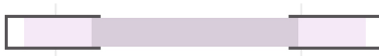
Figure 44: PlanningLine glyph [Aigner & Miksch, 2006]: the caps (the bracket-like forms at the far left and far right of the glyph) represent the earliest and latest starting shift and finishing shift; the maximum duration is indicated by the light gray area and the minimum duration is indicated by the dark gray area (see Figure 31).
