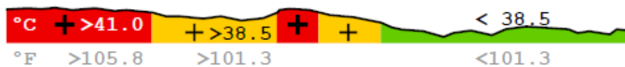
Figure 25: Qualitative - quantitative hybrid as used in Midgaard. The quantitative data of a fever curve is represented by the height while additional qualitative information is provided by the color-coding (critical fever values are colored red, moderate fever yellow and normal temperature green) [Bade et al., 2004].
