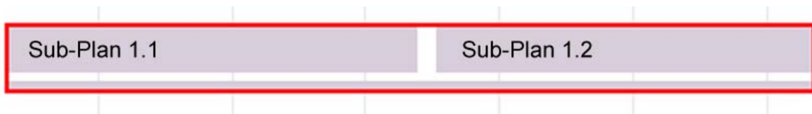
Figure 40: Sequential plan: the sub-plans are laid out on a timeline (x-axis) one after the other which shows that the plans are carried out in sequence.
