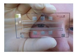
Figure 1: Photograph of the molecule chip, held by one of us (S.A.M.). The array of 1254, 10 μm diameter and 4 mm long electrodes extends over a total length of 50 mm. The electrodes run vertically, and are connected to either one of the six macroscopic pads to which the sinusoidal voltages are applied. (Photograph by Dr. Cynthia E. Heiner, FHI).
