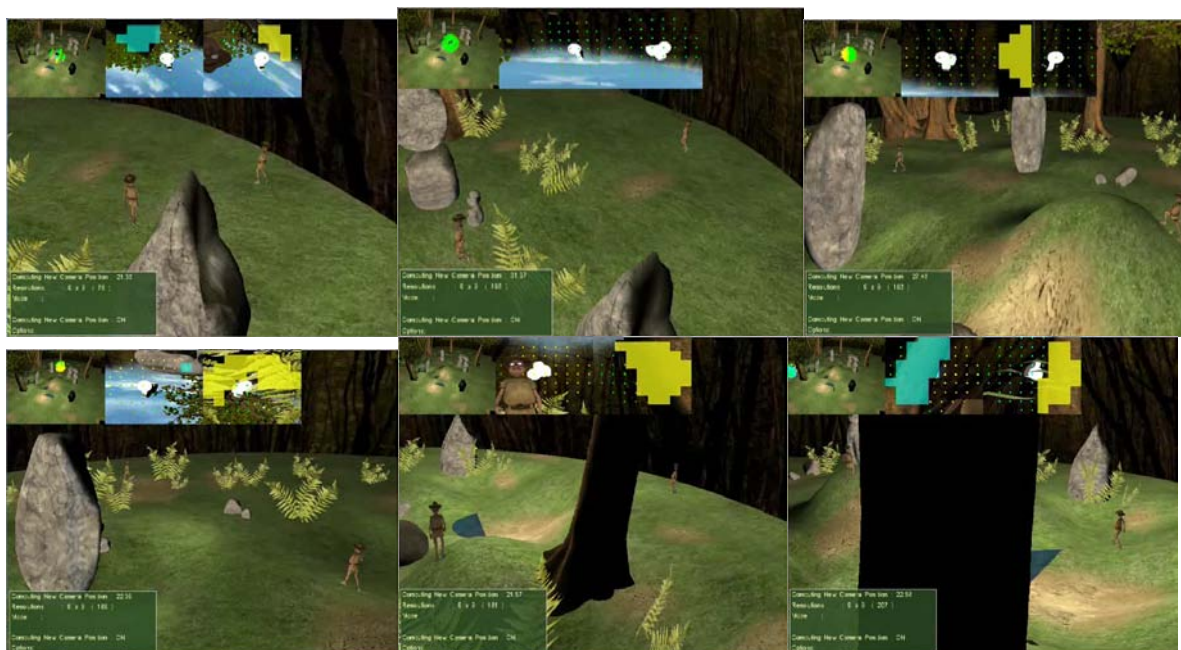
Figure 22: Simultaneous tracking of two characters in a complex 3D environment with both solid and sparse occluders, using a dynamic birds' eye view. The camera tracks both characters using the stochastic sampling to ensure an appropriate degree of visibility and temporal accumulation to ensure temporal coherence (avoid over-reactivity of the camera).
