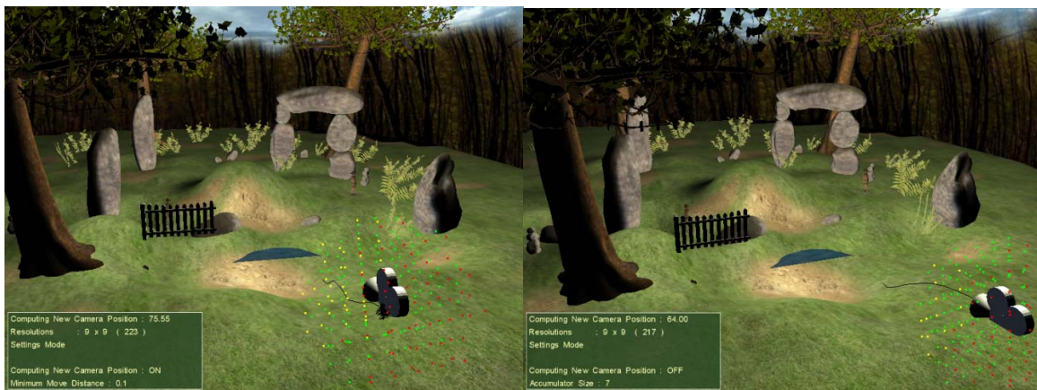
Figure 19 : Stability evaluation: a sparse occluder moves back and forth in front of two targets. The left figure shows significant movement by the camera (black knots at the basis of the camera), whereas the right frame shows how accumulating visibility states leads to significantly less camera movement.
