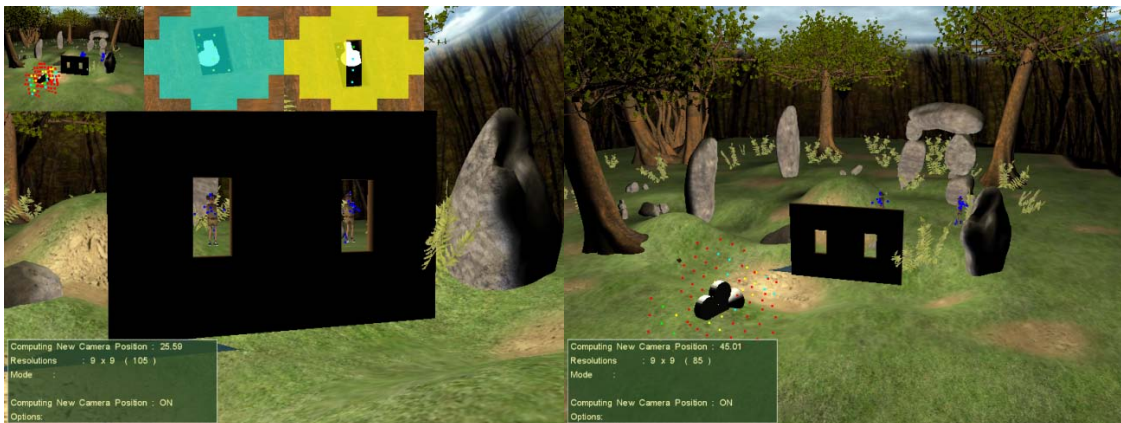
Figure 20 :Evaluation of the visual extent: each character presents a set of 10 target positions that have to be shot. The left view is a screenshot of the benchmark environment where camera configurations are displayed accordingly to their occlusion status: red if occluded for both characters, yellow or cyan if occluded for one of the characters, and green if unoccluded. The right view a subjective viewpoint taken from a solution camera configuration for which all 20 target points are in the shot.
