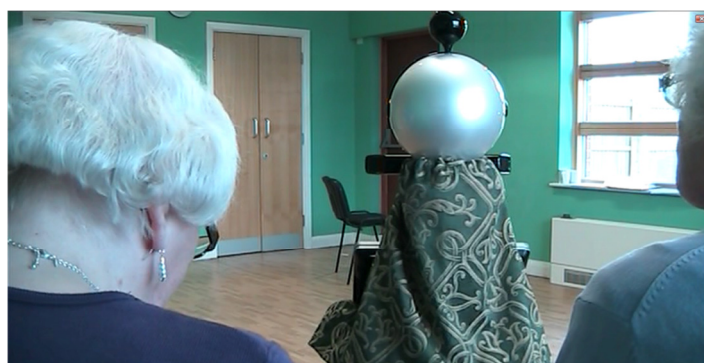
Figure 40 The ‘turn around’ command is useful, but the microphone is facing the wrong way
