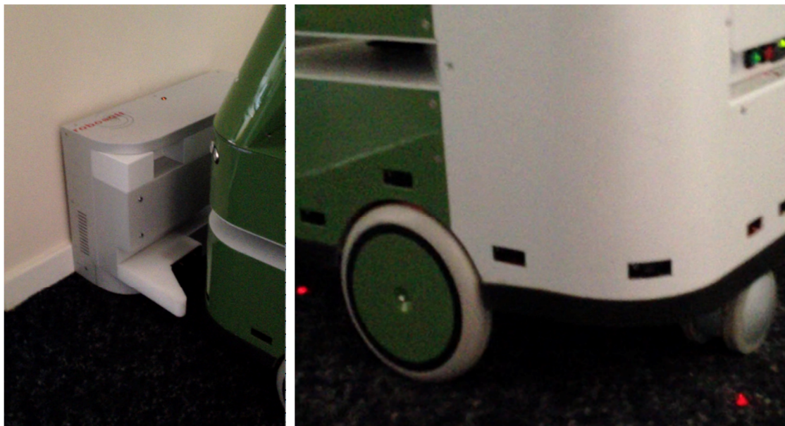
Figure 49 Even good alignment does not enable docking as back wheel is stuck in wrong position
