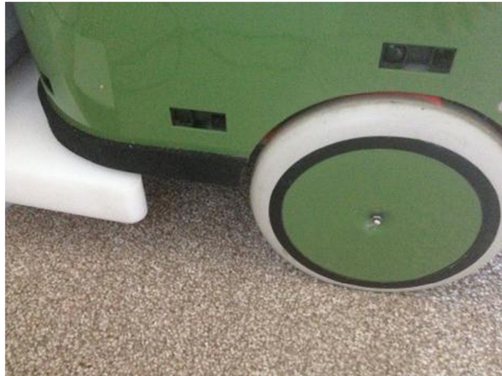
Figure 46 the robot sinks a bit and bumps into the white part of the charger instead of going over it
