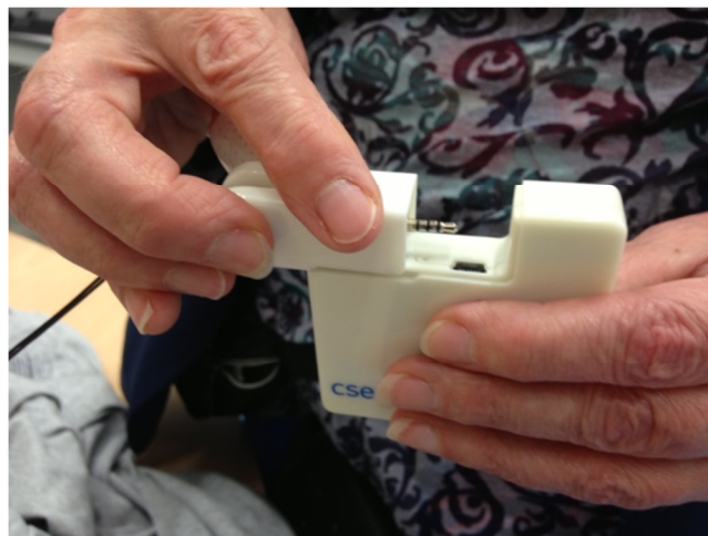
Figure 29 Connecting the data logger
