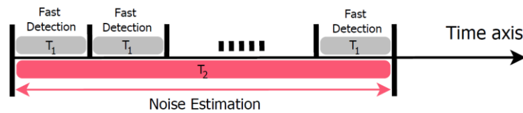
Figure 3-35: Trigger periods representation for short and long term (background) components
